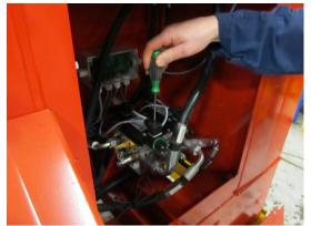
4. Release the contact as shown in the picture. Disconnect the cables from the contact.
