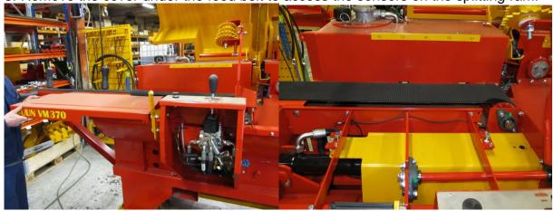
9. Remove the sensors for the splitting function. Mark, which is which, for properly installation. Distance from the sensor to the screw head for the plunger should be approx. 8 mm. Make sure the new sensors are fitted in the correct position for return and stop of the splitting ram. Check this by
