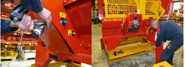
6. Release the switch and dismount the contacts as shown in the picture. Mark the contacts ensuring that these are connected correctly when new ones installed.
