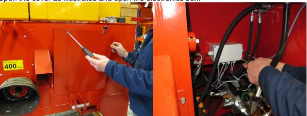
2. Open the cover aside the gear box. Untighen the screws holding the safety sensor. Release the safety sensor from the mounting bracket. Installing a new sensor, the distance from the safety sensor to the safety cover must be approximately 3mm.
