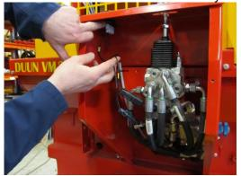
7. Open safety cover above the feed belt and loosen the screws for the covering lid as shown in the
