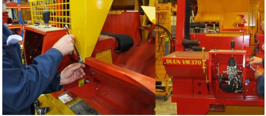
8. Remove the cover under the feed belt to access the sensors on the splitting ram.
