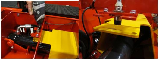
10. Release the contacts on the temperature sensor at the oil tank.
