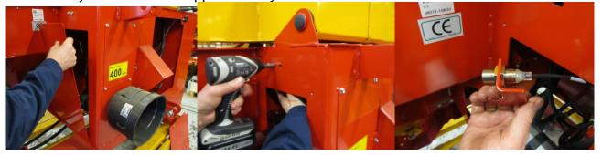
3. Release the contacts (4 pcs.) on the hydraulic control unit. Note carefully on the control panel where different functions are attached. The contacts are already marked originally.
